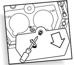
to insert the batteries, remove the battery compartment cover at the back of the game. (to remove cover, unscrew the cover, then push the cover in the direction of the arrow).
