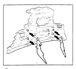
2 Press both supports onto back of assembled wall.
