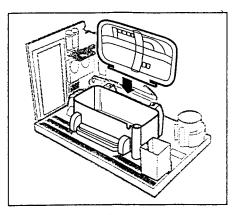
2 Insert one post on cover into edge of chamber, then snap other post onto edge of chamber.
