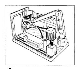
Insert bellows into holder. Press end of tube inside chamber. Fill chamber with cold water and ice cubes for best results. Pump bellows to produce bubbles.
