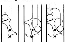
As a marble hits the bottom half of a gate it causes the gate to pivot as indicated by broken arrows. When several of the gates are loaded, one marble can set off an avalanche.
