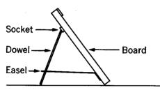
Insert the dowel through the hole in the easel. Lodge its upper end in the socket on the back of the board. Pull the easel down so that it is nearly horizontal when the board is standing.
