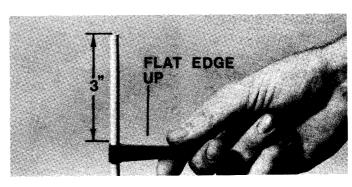
c. Place pointed tip on rod. d. Push weight into hand.
