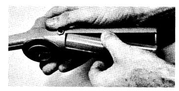
b. Insert 2 "D" batteries (not supplied) with the positive (button) ends facing the motor unit.
