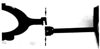
e. Place weathervane on top of rod.
