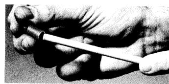
b. Insert rod with pointed end up into base #1.
