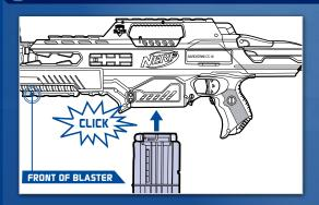
Insert CLIP into BLASTER (make sure arrow on CLIP points away from TRIGGER).
