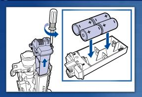
Phillips/cross head screwdriver (not included) needed to insert batteries. Loosen screws in battery compartment (screws remain attached to cover). Remove compartment. Insert 4 x 1.5V C alkaline batteries (not included). Replace compartment and tighten screws.
