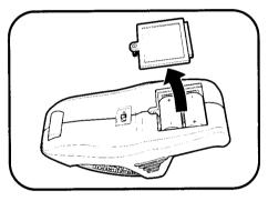
Whirlin' Vac is equipped with 2 "C" batteries. When the batteries are exhausted, use a Phillips screwdriver (not included) to loosen screw securing battery compartment door, and remove door. (Note: screw will remain attached to door.)
