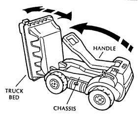
2. Lower handle into chassis. Lower truck bed onto chassis. Make sure latch locks truck bed in place.
