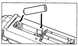
The + end of each battery must be inserted into the small, round, white plastic support, as shown.
