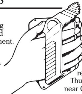
To hold, slide hand through handle. Fingers should be able to reach buttons. Thumb should rest near ON/OFF switch.
