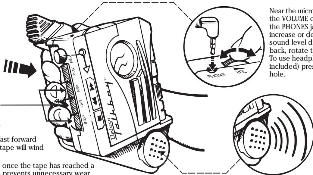
Near the microphone are the **VOLUME** control and the **PHONES** jack. To increase or decrease the sound level during play back, rotate the wheel. To use headphones (not included) press jack into hole.
