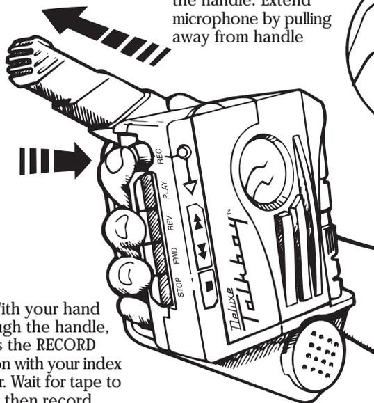
**3** With your hand through the handle, press the RECORD button with your index finger. Wait for tape to start, then record.
