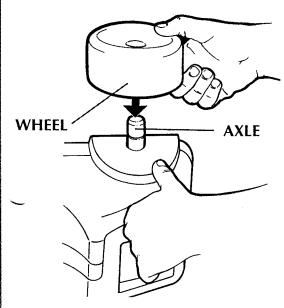
1. Attach the wheels to the 4 axles on the frame. Lie toy on its side, and push wheel onto end of axle until it snaps firmly into position. To prevent a pinch hazard, always keep fingers clear of area between wheel and axle. The wheel should spin freely on axle. If wheel does not spin freely, re-exert pressure and push wheel as far down onto axle as it will go. Repeat process for remaining 3 wheels.
