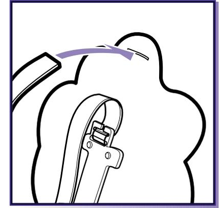
3. Facing front of hook, feed strap through top slot then bottom slot as shown.
