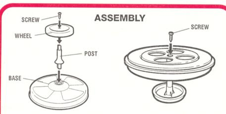
Remove screws that are attached to the bottom of the base. Push wide end of post into the top of the base. Attach wheel to the top of the post. Fasten wheel to post with screw.
