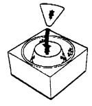
Place cone in dome, matching sun symbol on cone with matching symbol on inside of dome.
