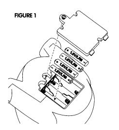
compartment. Be sure to match up the "+" and "-" symbols. Replace the door and tighten the screw.
