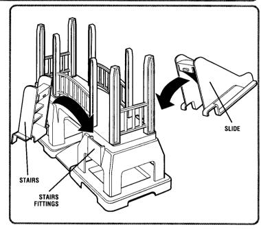
Assemble the slide and stairs into the 2 fittings of jungle gym as shown. Both the slide and stairs can fit into either of the 2 fittings.
