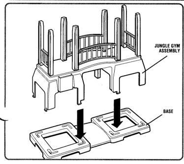
Snap the jungle gym assembly (with railings attached) to the playground base as shown. Either side of assembly can fit into either side of base.
