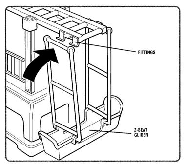
6. Attach the swing bars to the 2-seat glider swing, then fit top of bars into fittings on other end of monkey bars.
