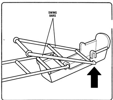
5. Attach the swing bars to the 2 seat- glider swing.
