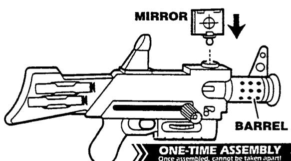
With barrel pointed straight forward, line up mirror as shown. Snap mirror into place.
