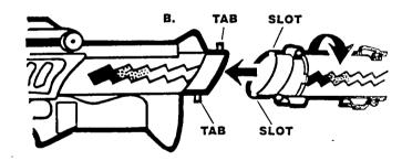
7. Barrel can be snapped on top of base unit to be used as a scope (A). To extend length of base unit (B), align slots on one end of barrel with the tabs on the base unit. Insert and turn as shown until you hear a click. Barrel can be removed by reversing the procedure.
