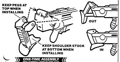
Attach stock to rear of base unit by spreading the two pegs apart, then inserting and snapping them into the holes as shown. Stock folds out and in.
