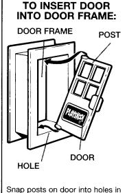
Snap posts on door into holes in top and bottom of door frame.
