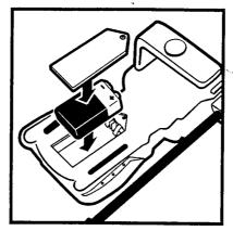
Insert one 9-volt battery (alkaline recommended) into compartment as indicated.
