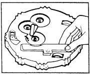
3. Replace the battery cover. With the batteries in place, set the battery cover back into its original position. Replace the screw.
