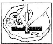
1. Turn the platform over. Remove the battery cover. Using a small phillips screwdriver, carefully loosen the screw holding the cover in place. The cover can easily be lifted off with the screw.
