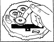
Removing a skating disc. To remove a skating disc. place forefinger under skating disc and carefully lift off.
