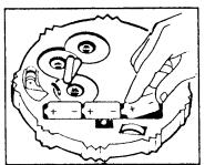
2. Place 3 size "C" Alkaline batteries inside the battery chamber.
