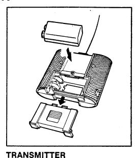
Insert one 9-volt alkaline battery.
