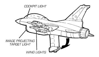
When firing handle is pulled down the wing lights, cockpit light, jet sounds and image projecting target light are activated.
