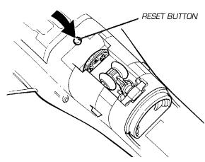
4 Jet projector light will automatically shut off after approximately 41/2 minutes. Press reset button to reactivate projector light. When using jet outside or in bright light, we recommend leaving projector light off to conserve battery life.
