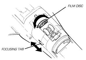
**2** By turning the film disc you can choose the target image to be projected. Adjust the image with side focusing tabs as shown. For best projection results, you'll need a room that's dark. Project image onto a wall from 6 to 8 feet away.
