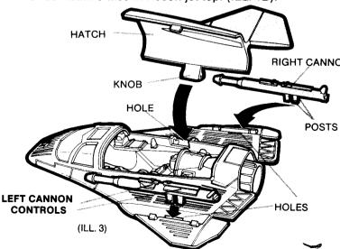
Insert posts on left and right cannons into holes in outer wings. **Note: Cannon controls face outward.** Do not force cannons into holes. Fit knob on hatch into hole on side of Recon jet and snap other knob into place. (ILL. 3)
