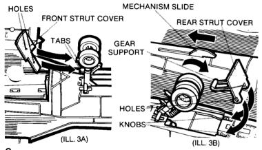
3 A Snap holes in front strut cover over tabs on front strut. (ILL. 3A)
