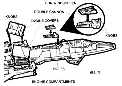
Fit front knob on left engine cover (marked "L") into hole in left engine compartment. Snap rear knob into place. Repeat with right engine cover (marked "R"). Insert post on gun windscreen into hole in double cannon (see inset). Snap knobs on double cannon into holes in fuselage. (ILL. 7)
