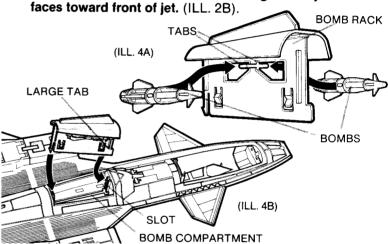
A Fit bombs over tabs on each side of bomb rack.
