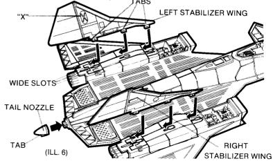
6 Turn Raven right side up. Insert tabs on left stabilizer wing (marked "X") into wide slots in left wing. Slide. wing back and snap into place. Repeat with right stabilizer wing. With tab down, fit tail nozzle over knob on jet tail. (ILL. 6)
