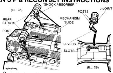
A Turn jet upside down. Make sure mechanism slide is in forward position. Insert 2 rear strut levers into holes in mechanism gear, making sure "shock absorbers "face toward front of jet. Snap posts into slots. (ILL. 2A). B Repeat with front strut lever, making sure L-joint
