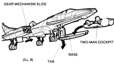
8 Lower landing gear by sliding gear mechanism forward. Push tab forward and pull down to lower cockpit base. Fittwo-man cockpit into base. Two-man cockpit is removable for loading. (ILL. 8)
