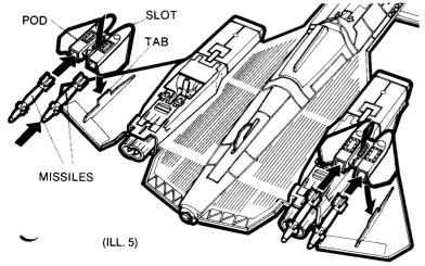
Insert missiles into missile pods as shown. Fit slots in missile pods over tabs on outer wings. (ILL. 5)
