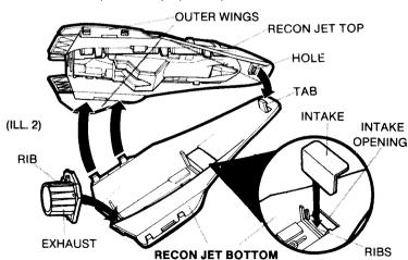
With intake vents facing opening in RECON JET BOTTOM, fit intake between ribs and snap into place (see inset). With rib on top, fit exhaust into slot in recon jet bottom. Insert front hole in Recon jet top over tab on Recon jet bottom. Press outer wings to snap side tabs into place. (ILL. 2).
