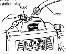
2. After filling the tank with water, your child can squeeze the pump handle to squirt water. It will take about 10 squeezes to draw the water through the hose and into the handle. Note: We suggest that you place the pump handle on the holder when it's not being used. If you leave the pump handle on the ground, the water will drain from it and empty the tank.
