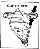
4. Press clip halves together, leaving one end unfastened. Open clip halves to allow folded part of bag to fit between clip halves. Press the unfastened end of clip halves together so that clip locks onto bag.
