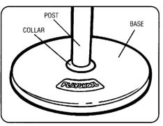
Align tabs on post with slots on base and press into place. Post is positioned properly when collar is flush with base as shown. Note: If post won't press into place, rotate base until proper alignment is achieved.
