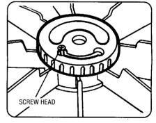
4. Align metal tabs on battery door with slots in battery compartment. Screw head should fit through opening in battery door as shown.
