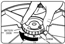
5. Press and rotate battery door in a clockwise direction until opposite end of opening aligns with screw. (Note: If battery door doesn't rotate, screw hasn't been loosened enough. Make sure screw head rests above opening in battery door.) Tighten screw to hold battery door in place.
