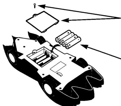
**1** Remove screw. Remove battery door from bottom of vehicle as shown.
