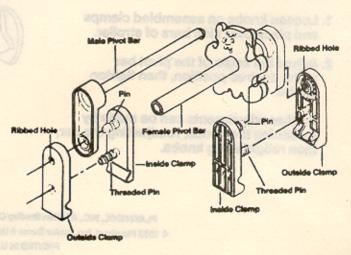
2. Screw a knob onto each threaded pin as shown.
