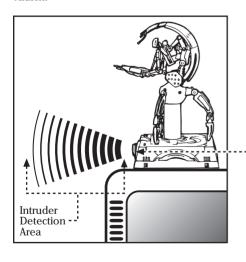
Set on table or other flat surface. Turn so --- Heat Sensor Lens faces desired Intruder Detection Area.
