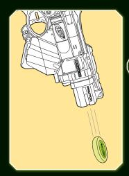
Point the blaster at the ground. The jammed DISC will fall out.
