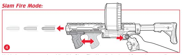
Hold trigger down, and rapidly slide Slam Fire Handle back and forward repeatedly. **Be sure to slide handle** all the way back and all the way forward to prevent **damaging darts.**
