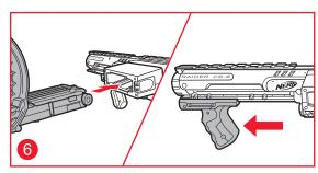
Once jam is cleared, replace Drum Magazine and slide Slam Fire Handle forward. This should load another dart.
